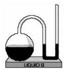
The images to the left show two manometers in which liquid A has a higher vapor pressure than liquid B.
