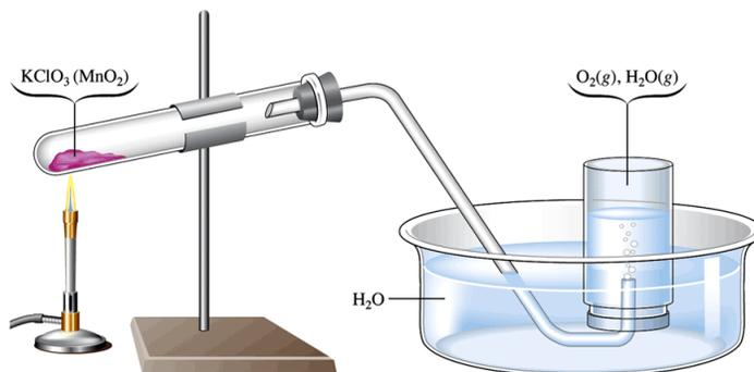
**Example:** A sample of solid potassium chlorate ( $KClO_3$ ) was heated in a test tube and decomposed by the following reaction:  $2KClO_3 \rightarrow 2KCl + 3O_2$
